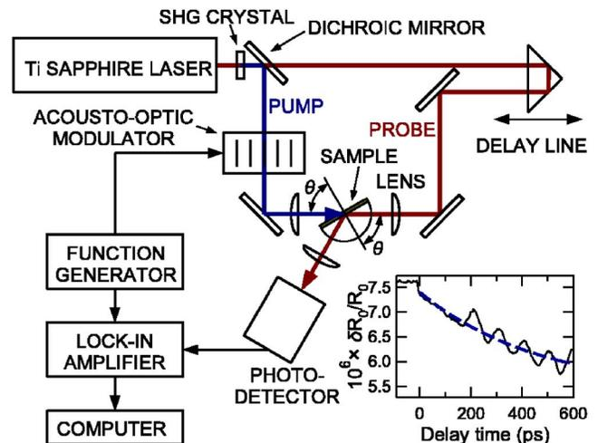
FIG. 1. (Color online) Experimental setup. Inset: relative reflectivity change for  $\theta=60^\circ$  (solid line) and exponential fit to thermorefectance (dashed line). SHG: second-harmonic generation crystal.
