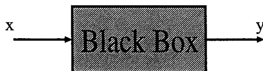
Figure 1.1: The black box. Input x vs. output y relations of the box is determined by a conditional probability p(y|x; \theta) .
