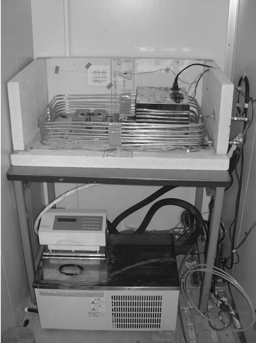
Figure 4 Complete view of test apparatus, including the surrounding insulation box
