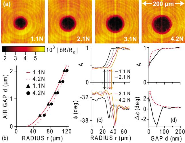
FIG. 3. (Color online) (a)  $|\delta R/R_0|$  images of the contact. (b) Measured air gap ( $\blacktriangle$ ,  $\bullet$ ) and Hertz theory (lines) for two loads. (c) Normalized amplitude and phase for  $t = -10$  ps. Arrows: contact radii. (d) Normalized amplitude and phase difference for 1.1 N and 3D thermal-diffusion theory (dashed lines).
