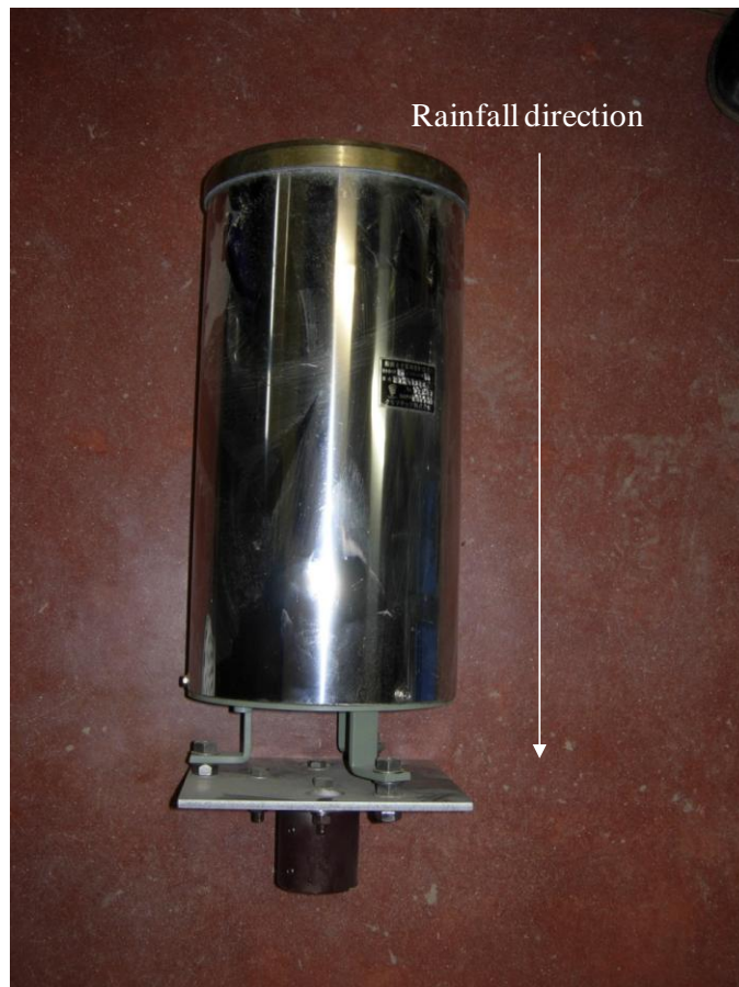
(f) Rainfall gauge
