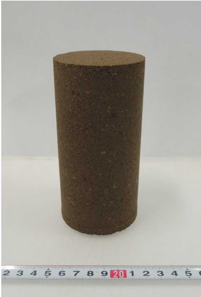
(a) K soil, D_s = 70 mm, Optimum water content condition, 11 blows per a layer
