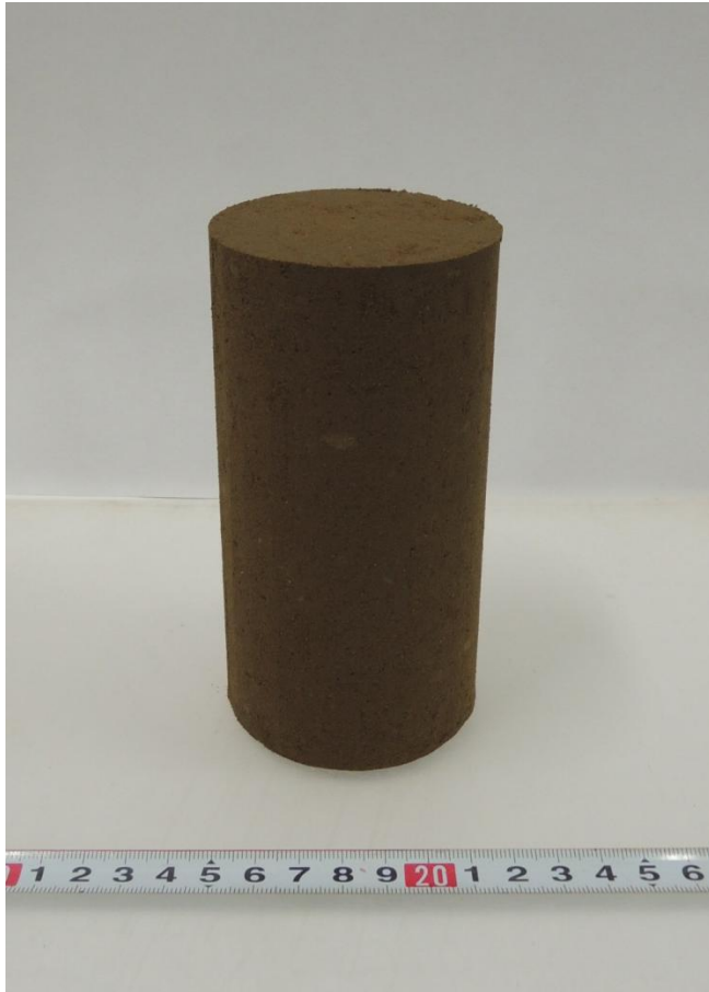
(a) I soil, D_s = 70 mm, Optimum water content condition, 25 blows per a layer
