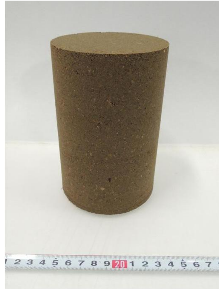
(b) K soil, D_s = 100 mm, Optimum water content condition, 25 blows per a layer
