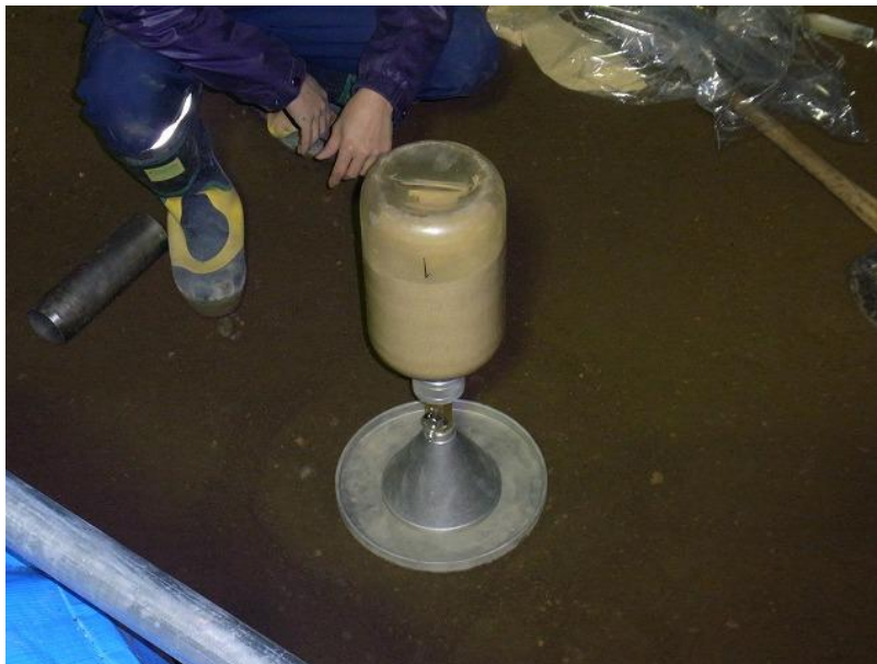
(f) Conducting sand replacement method
