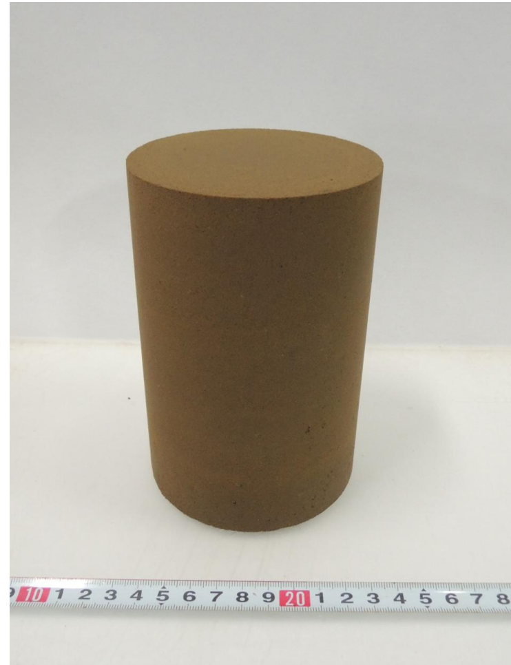
(b) I soil, D_s = 100 mm, Optimum water content condition, 25 blows per a layer
