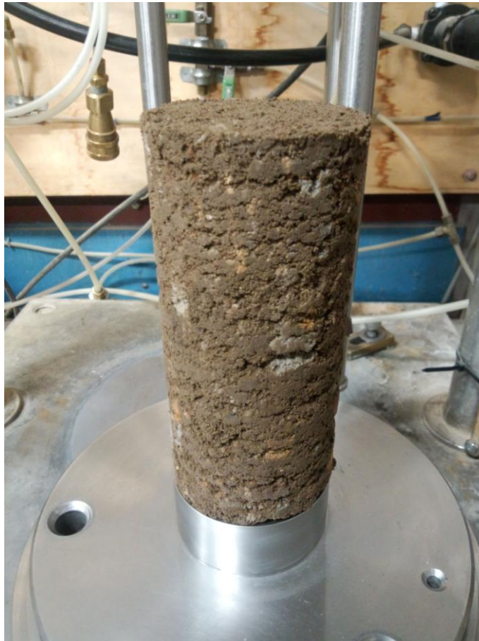
Photograph 4.1.9 K_{\text{original}} specimen for liquefaction test sampled by thin-wall sampling from FE-2012; w_i = 42.2\% , D_{ci} = 91.0\% (see 4.2 Testing on full-scale embankment )
