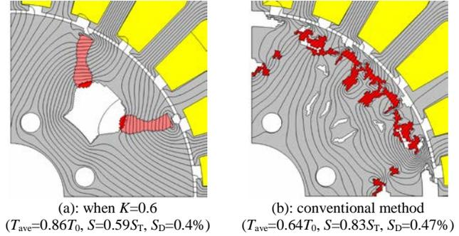
Fig. 12. Resultant rotor shapes obtained by different settings.
