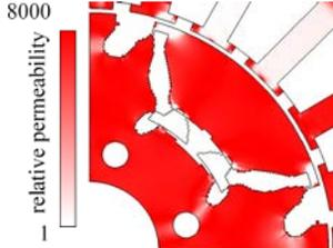
Fig. 11. Permeability distribution in rotor core for (A).
