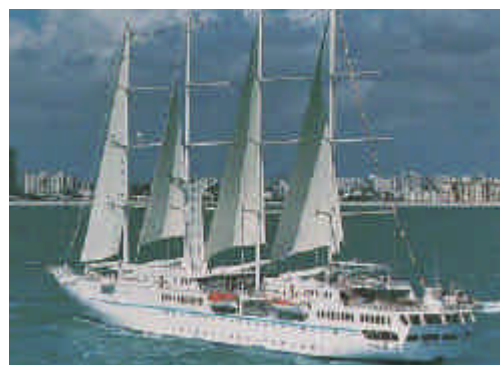
Fig.3 Modern sail-equipped cruising ship “Wind Star” (GT:5703, Sail area:2005m 2 )
