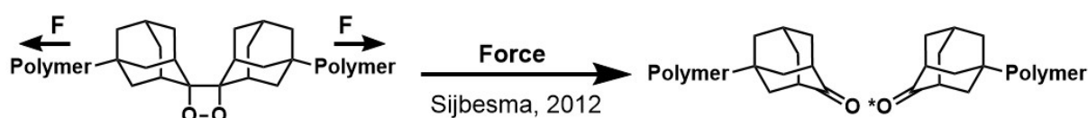
Figure 1-3. Activation of 1,2-dioxetane based mechanophore.
