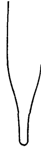
Text-fig. 1. Diagram of bottle-shaped glassware for the detection of equine Day-6 and Day-7 embryos. It is 10.5 cm at the top and 2.8 cm at the bottom in outside diameter and 41 cm in height. The capacity is about 1500 ml.
