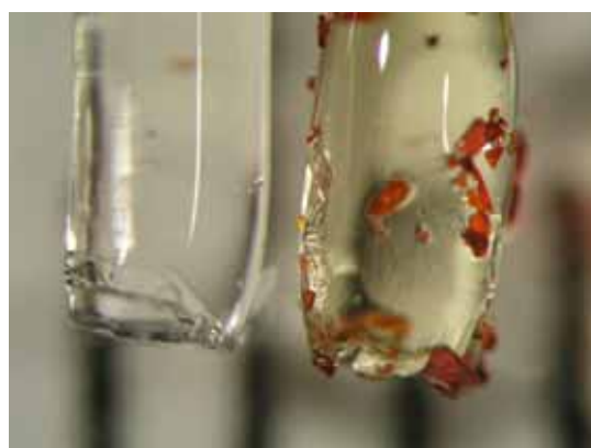
Figure 1. Cylindrical NIPA-PMDDP gels with (right) and without (left) oil-soluble dye Yellow AB. Fine crystals of Yellow AB are attached to the gel in the right side figure.
