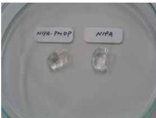
Figure 2. NIPA-PMDP (left side) and NIPA (right side) gels after immersing in water containing Yellow AB powder
