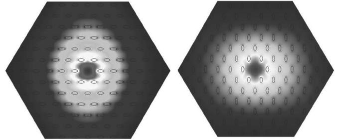
Fig. 4. Normalized intensity distributions of the fundamental mode calculated at maximum thermal sensitivity and for operational wavelength of  $\lambda = 1550$  nm, for type-A PCF (left panel) and type-B PCF (right panel). The total number of air-hole rings is six for both cases.
