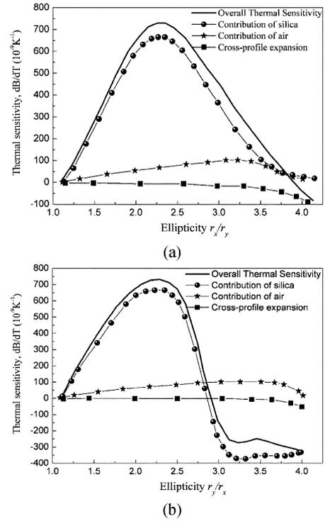
Fig. 2. Contributions of silica (circles), air (stars), and the cross profile expansion of the geometry (squares), to the overall thermal sensitivity ( $\text{K}^{-1}$ ), at  $\lambda = 1550$  nm, as a function of the air-hole ellipticity- $e$  for (a) type-A PCF and (b) type-B PCF. For both cases, the maximization of the sensitivity function occurs for an air-hole ellipticity value of  $e = 2.27$ .
