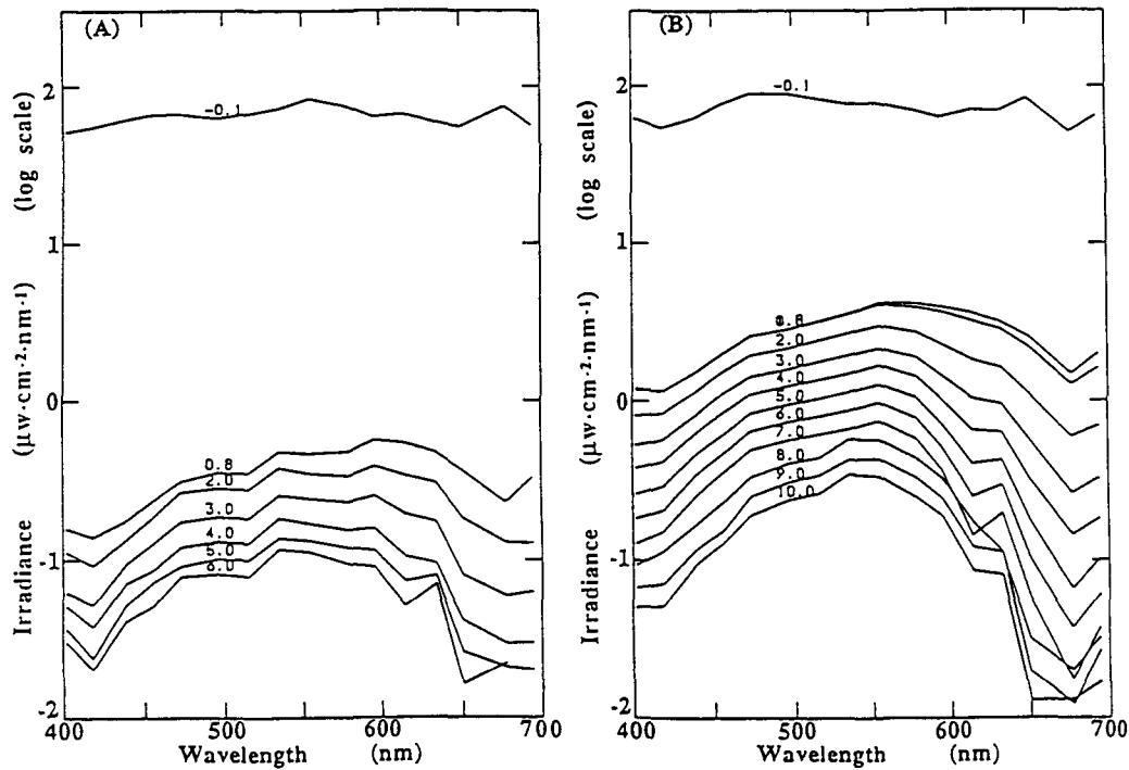
**Fig. 3.** Downward spectral irradiance measured under sea ice on February 22, 1992.
