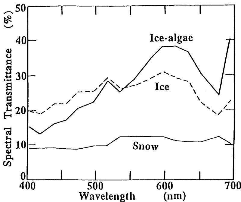
**Fig. 6.** The transmittance of the layers of surface snow, upper sea ice (Ice), and bottom sea ice (Ice-algae) including ice algae
