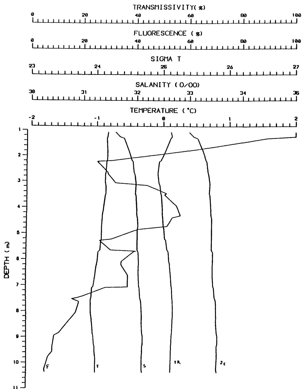
Fig. 16. Vertical profiles of temperature (T), salinity (S), sigma-t ( $\sigma_t$ ), transmissivity (TR), and fluorescence (F) at 1606 hr on March 21, 1992
