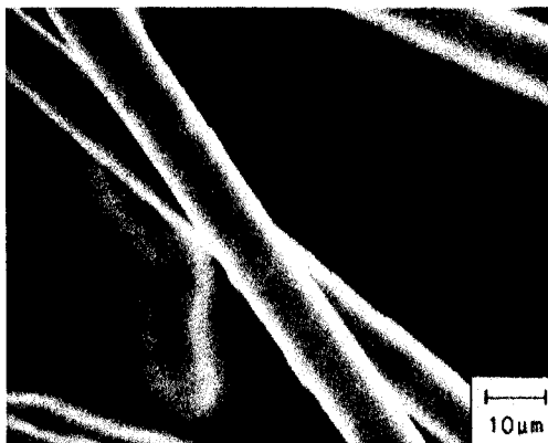
Fig. 5-3 SEM Micrograph of VGCFs (Carbon Source: n -Pentane)
