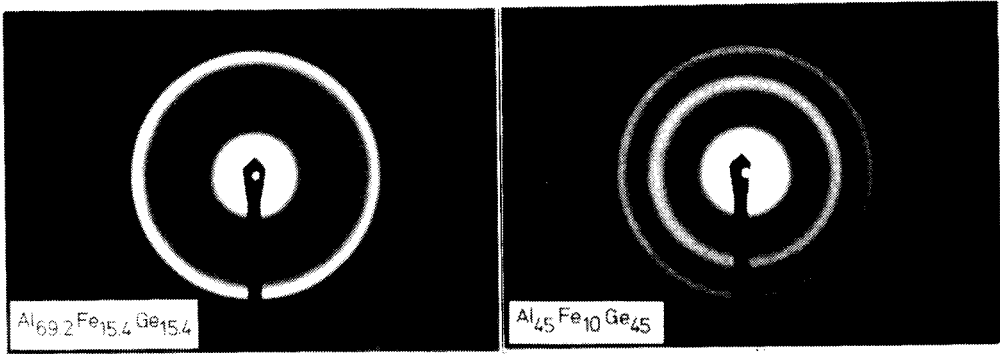
Fig.3-18 Selected area diffraction patterns of \text{Al}_{69.2}\text{Fe}_{15.4}\text{Ge}_{15.4} and \text{Al}_{45}\text{Fe}_{10}\text{Ge}_{45} amorphous alloys.
