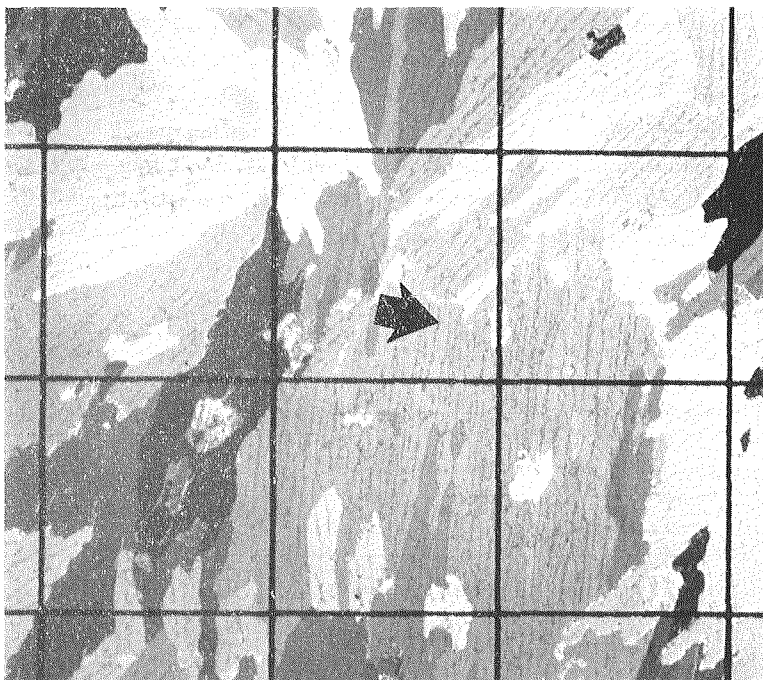
Fig. 8. Horizontal thin section enlarged to show grain and subgrain structure. The grid is 1 cm on a side
