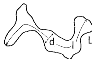
Fig. 6. Definition of l and d for the ice grain
