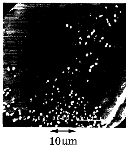
FIG. 1. SEM picture of a photoetched surface of single-crystalline GaAs.
