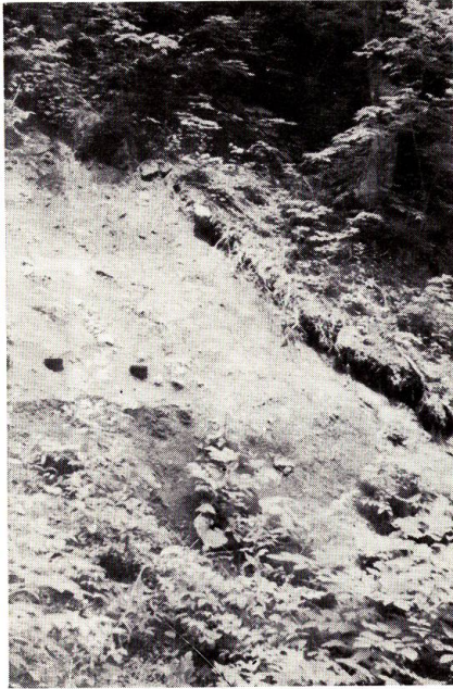
I) Infiltration test plot No. 4 on SE failure slope at Asshinai, Amano-kawa River Basin, ( f_c = 224 \text{ mm/hr} ). 天の川流域アツシナイにおける南東面崩壊地の No. 4 滲透試験区
