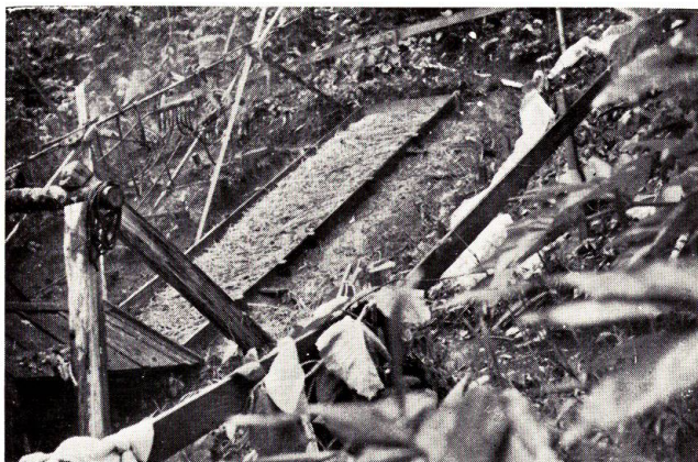
I) Test, No. 57-7, of simulated rainfall with intensity of 189 mm per hour on No. 6 b covered with Timothy grass (10 cm depth).
