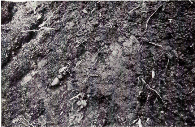
I) Test, No. 56-10, showing the erosion pavement after the end of rainfall with intensity of 416 mm/hr.
