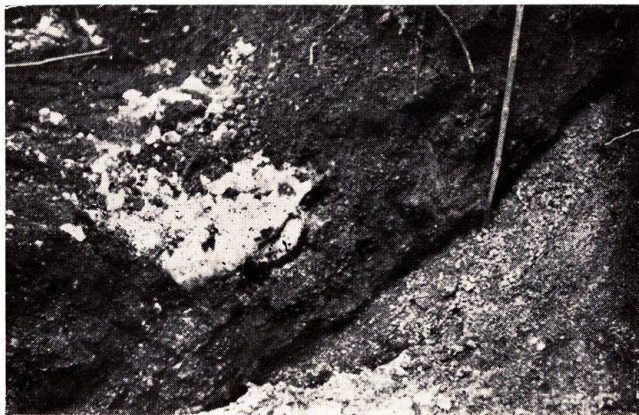
III) Ditto, residual concrete frost in the bottom of contour furrow. (Frost depth: 25~27 cm from soil surface)
