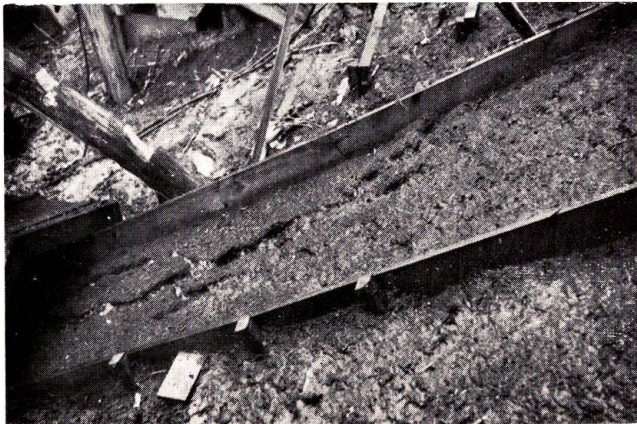
II) Ditto, development of rill erosion after 36 minutes from beginning of rainfall.
