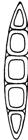
Fig. 10. Schematic drawing of a wood ray in tangential sectional view. The ray consists of ray parenchyma cells of round outline in cross section.
