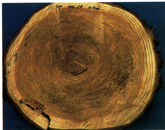
Photo 3. Cross section of a Japanese larch log showing the brown cubical rot caused by Sparassis crispa at a height of 0.3 m above the ground.
