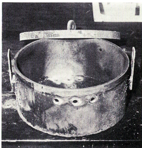
Photo 2. A vessel made of iron for carbonization.
