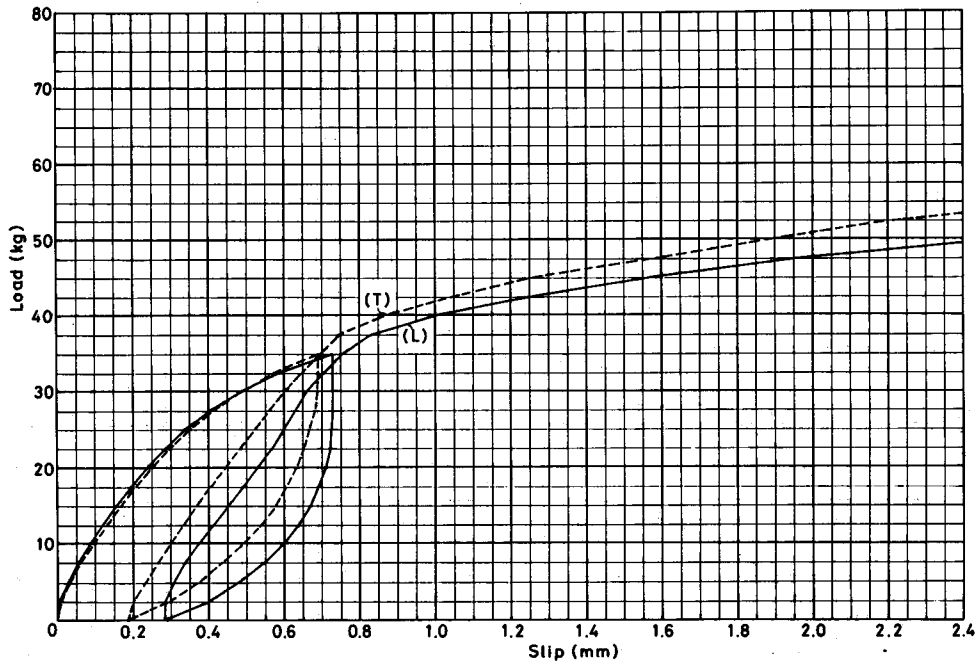
Fig. 3. Effect of the grain direction of main-member.
