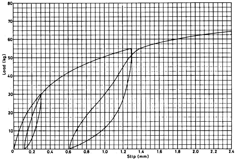
Fig. 5. (1) Basic load-slip curve of a nailed wood-plywood joint with a CN50 nail. (Ezomatsu-todomatsu 204 and Kapor 7.5 mm plywood)
