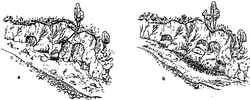
Fig. 13. Illustration of channel response to landslide debris in the torrential river.
