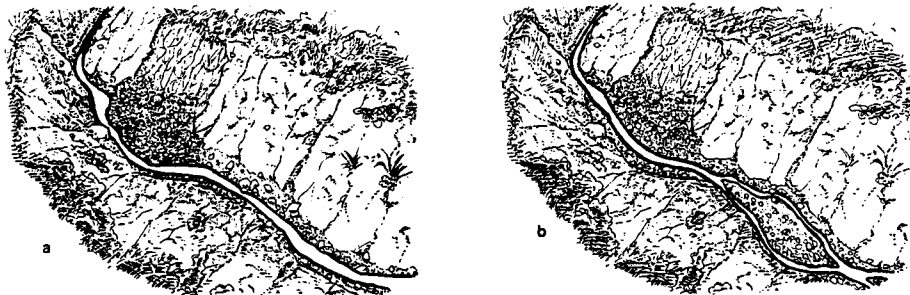
Fig. 14. Illustration of channel response to landslide debris in the placid stream.
