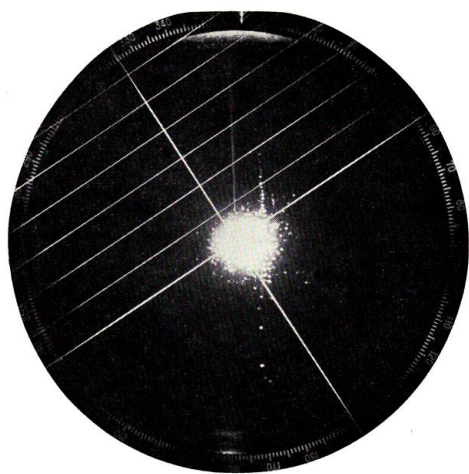
Fig. IV-2-a. Echo images on the P.P.I. scope showing flag floats and corner reflectors mounted on long-lines.
