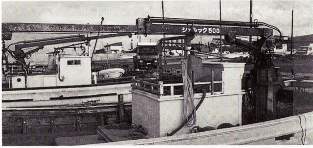
Fig. 3. Hydraulic crane on a scallop-aquaculture boat.
