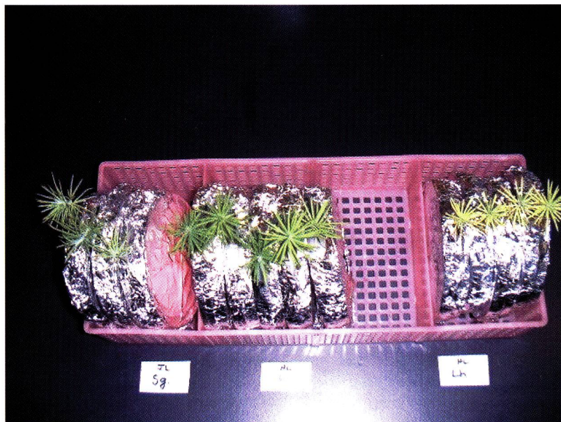
Fig. 2. Aseptic synthesis of ectomycorrhizae. Tree seedlings growing in petri dishes placed in plastic box inside a growth cabinet.
