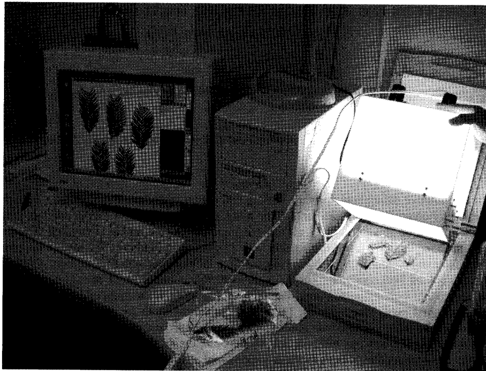
Fig. 1. The light-box-scanner system for measurement of projected (silhouette) area of three-dimensional material. A light box containing two 23-watt fluorescent bulbs (each equivalent in brightness to 100-watt filament bulbs) is placed atop the scanner bed to uniformly illuminate the background and eliminate shadows. Images were scanned at maximum contrast to obtain the projected (silhouette) area measurement.
