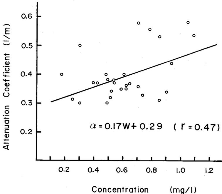
Fig. 3 Relation between attenuation coefficient and concentration of suspended matter
