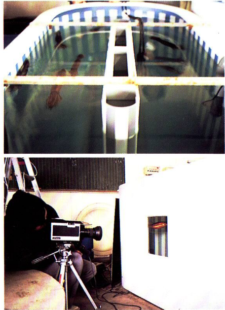
Fig. 2. Experimental set-up for squid swimming speed observation. The major radius, minor radius, and depth of the oval-shaped aquarium tank are 1, 0.5, and 1 m, respectively.
