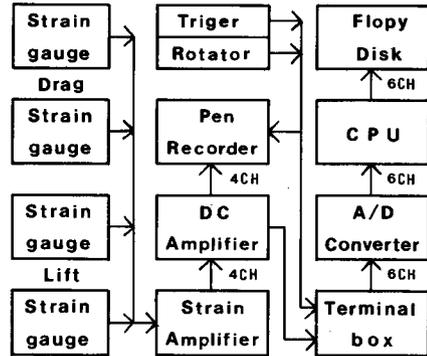
Fig. 2. Measuring system of aerodynamic forces.
