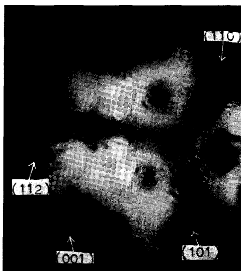
Plate 8. After several flash at 3000°K, i=4.0 \mu A and V=8000 volts.
