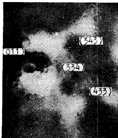
Plate 6. After heat treatment at about 1950°K for 10 minutes, i=0.5 \mu\text{A} and V=7600 volts.
