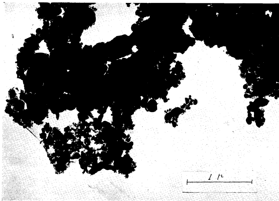
Fig. 4. The catalyst particles transferred onto carbon film. \times 36,000
