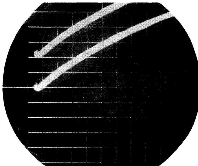
Plate 11. The potential-time variation after switching on a polarizing current on Pt in aqueous 0.1 N Na 2 SO 4 , pH 8.3, i = 1 \cdot 10^{-3} mp., 1 mv/Div, 10 \mu sec/Div.
