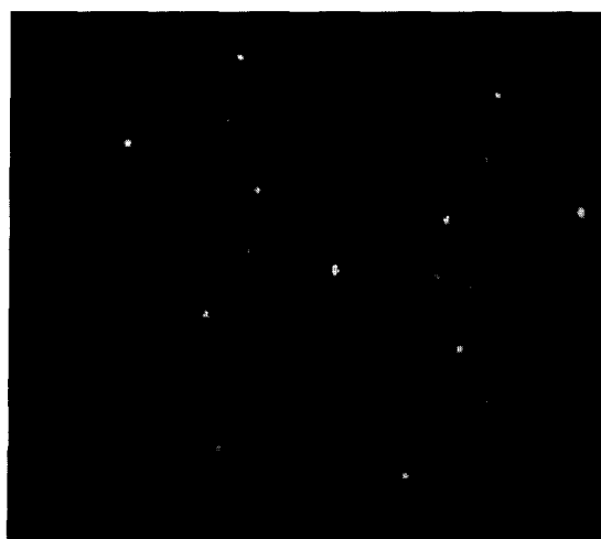
Fig. 11 a. LEED pattern of the \begin{vmatrix} 2 & -1 \\ 2 & 4 \end{vmatrix} surface structure obtained after heating the NH 3 covered Fe-3(111)x(110) to ~700 K (72 eV).
