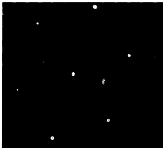
Fig. 3 a. LEED pattern of the (2 \times 2) + \begin{vmatrix} 1 & -1 \\ 1 & 2 \end{vmatrix} surface structure obtained after mild heating the \text{NH}_3 covered \text{Fe}(110) - (2 \times 2) which undergoes LEED beam effect (80 eV).
