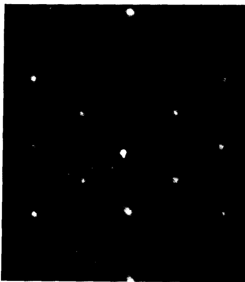
Fig. 1. LEED pattern of the (2 \times 2) surface structure obtained after chemisorption of NH 3 on the Fe(110) at \sim 273 K and then flashing to \sim 310 K (82 eV).
