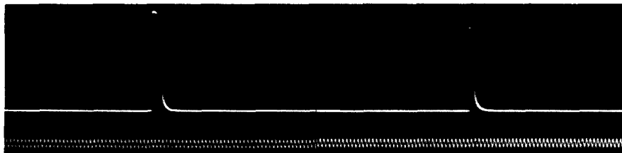
Fig. 1. Cathode ray oscilloscopic records showing the time course of the flash of light from the xenon stroboscopic photography lamp (Kako S-2), obtained with a phototransistor. Time mark: 1000 c.p.s.
