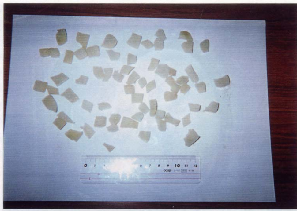
Photo. 6-4. Sponge particles used in the second cleaning.
