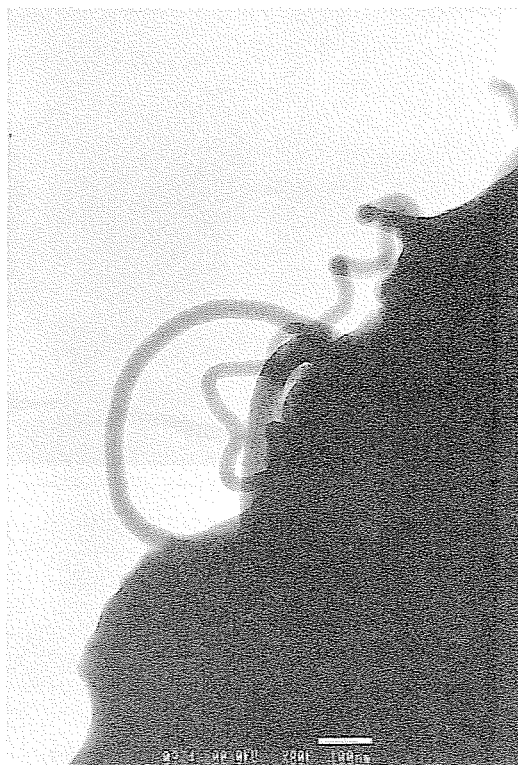
Figure 5.7. TEM micrograph of CNFs grown from Pd/Ni catalyst.
