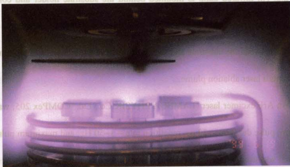
Figure 2.2. A photograph of RF plasma and a laser ablation plume at an Ar gas pressure of 500 mTorr.
