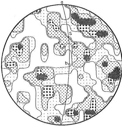
Fig. 13-i Specimen 9 , 300 quartz [0001] axes from banded gneiss Contours 2.5-2-1.5-1%
