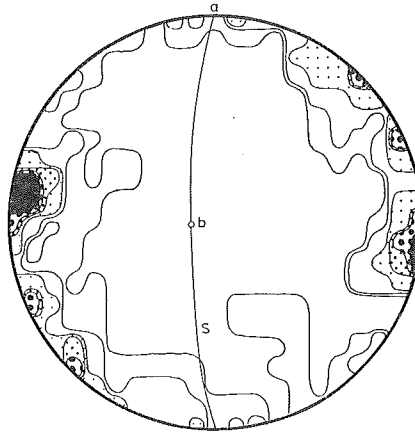
Fig. 15-h Specimen 8 , 100 cleavage poles of muscovite from banded gneiss Contours 10-8-6-4-2-1%.
