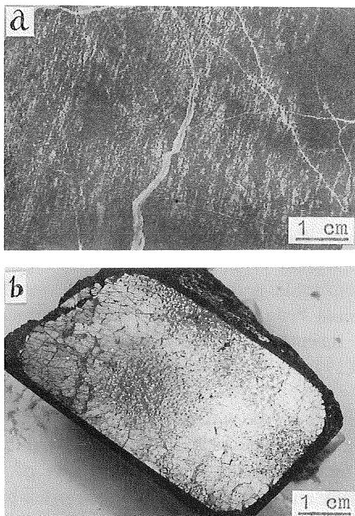
**Fig. 2** Photographs illustrating two kinds of chromite ore.
