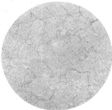
Photo. 2 (a) Outside. Weight 10gr, sulphur content 0.2%, temp. 1196°C.
