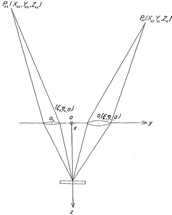
Fig. 9. Representation of detection process in which two apertures are used and are translated so that the images remain fixed as the angle of incidence changes.
