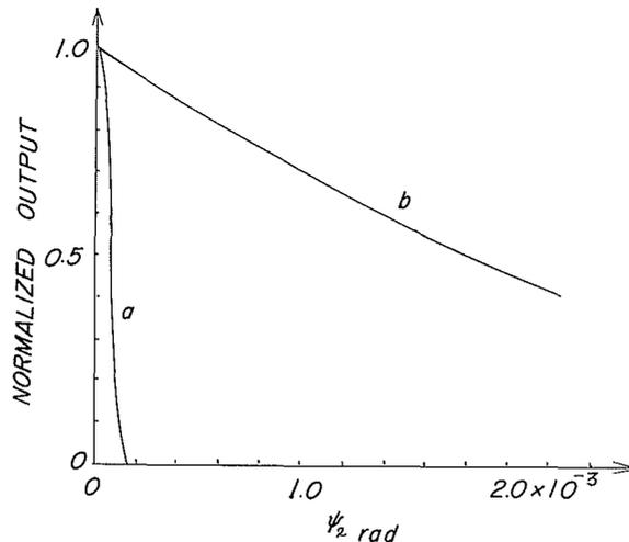
Fig. 11. The theoretical normalized output  $[D(\psi_2)/D(0)]^2$  vs  $\psi_2$  in the case where  $\theta_1 = \varphi_1 = \pi/2$  and  $\delta_2 = 0$  at  $6328 \text{ \AA}$ ; (a) unfocused light on the rectangular detector of sides  $a = b = 0.4$  cm, and focused light with a single aperture of sides  $\xi_0 = \eta_0 = 0.4$  cm and  $s' = 65$  cm, (b) focused light with two apertures of  $\xi_{a1} = \eta_{a1} = \xi_{a2} = \eta_{a2} = 0.4$  cm and  $\lambda_1 = \lambda_2$ .
