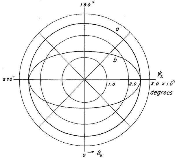
Fig. 5. The angular selectivity of  $\delta_2$  and  $\psi_2$  for  $D(\theta_1, \theta_2, \varphi_1, \varphi_2) \geq 1/\sqrt{2}$  in the rectangular photosensitive surfaces at  $\lambda_2 = 1 \mu$  and  $\theta_1 = \varphi_1 = \pi/2$ ; (a)  $a = 1 \text{ cm}$ ,  $b = 1 \text{ cm}$  (b)  $a = 1 \text{ cm}$ ,  $b = 2 \text{ cm}$ .
