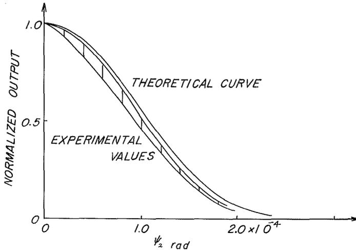
Fig. 13. Detected signal for unfocused light vs angular mismatch in the case in which the radius of the circular photosensitive surface is 1.5 mm and  $\theta_1 = \varphi_1 = \pi/2$  and a MS9S photomultiplier is used.
