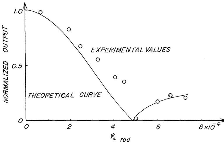
Fig. 14. Detected signal for unfocused light vs angular mismatch in the case where the rectangular photosensitive surface of sides  $a = 1.3$  mm and  $b = 2$  mm,  $\theta_1 = \varphi_1 = \pi/2$ ,  $\delta_2 = 0$  and a 7696 photomultiplier is used. (From Mr. K. Koyanagi).
