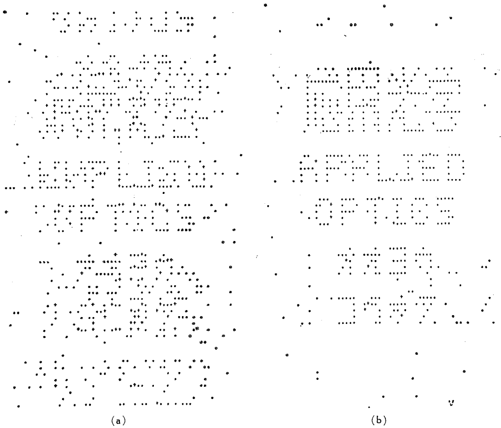
Fig. 15. Numerically synthesized images, where a is due to one array function and b is the intensity average of six images which are synthesized by the temporal array describing six different array functions obtained by the procedure of Fig. 14.
