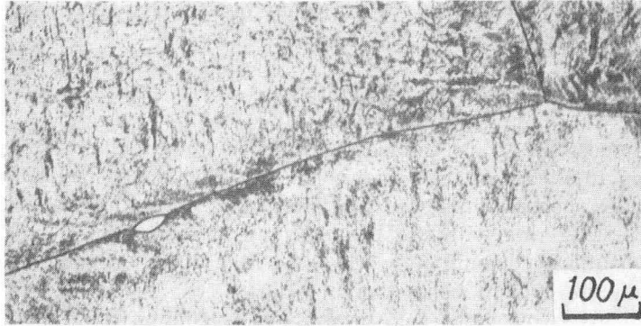
Photo. 1. Dislocation pile-ups along grain boundary produced by cold rolling. Aged at 200°C for 10 hr and etched with Morris etchant.
