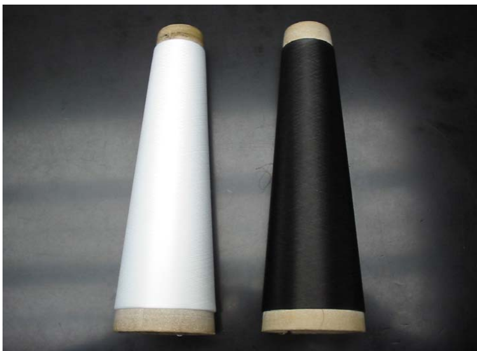
Fig. 3. Photos of the polyester multifilament yarns before (left-photo) and after (right-photo) being dye-printed with the CNT-based dyestuffs. The yarns were about 10,000 meters long.
