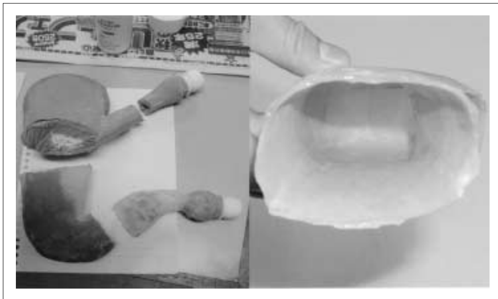
Fig. 4 Cutting the mold and removing the clay.
