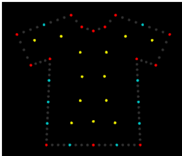
Fig. 4 Yellow nodes indicate the inserted interior nodes using magnet based method.
