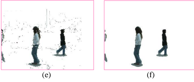
Fig. 2 Results of foreground mask. (a) Background image. (b)The frame contained foreground. (c)The result of background subtraction is derived from using RGB color model. (d) The result of noise removal (c). (e) The extracted foreground by proposed method in YCbCr color model. (f) The result of noise removal of (e).
