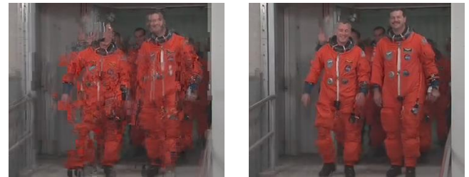
(a) Frame copy (b) Proposed Fig. 8. Comparisons of the subjective quality of the 53 th frame on Crew sequence under 20% packet loss ratio.
