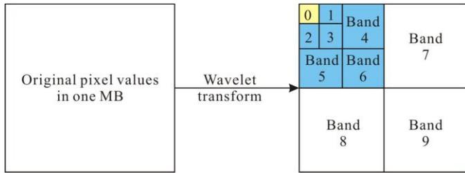
Fig. 3. Three-level wavelet transform of the block.
