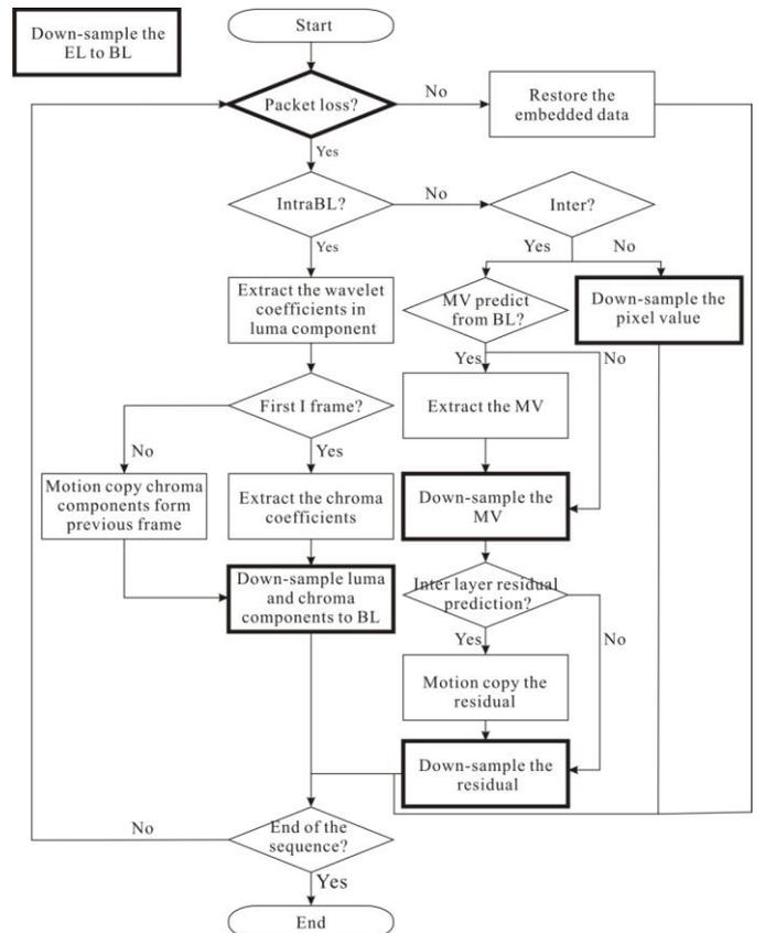
Fig. 5. Flowchart of the proposed scheme in decoder
