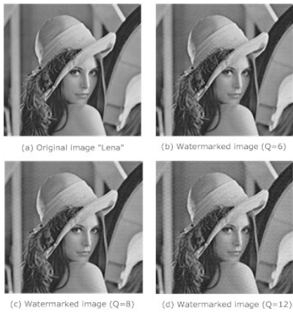
Fig. 5. Demonstration of the invisibility for Lena. PSNRs of (b), (c) and (d) are 41.92, 39.55 and 36.05 respectively.
