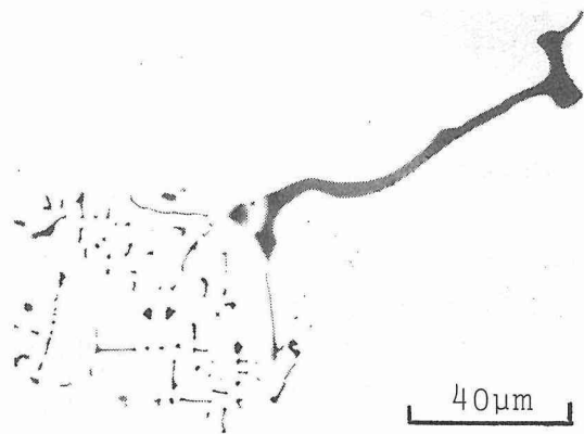
Photo. 2 Type II MnS coexisting with residual molten steel.
